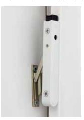
When setting down the window sash on turn-only and tilt-and-turn windows gradually, the MULTI-Vent tilt restrictor allows you to select the opening angle freely. The integrated braking effect means that the sash stops at the desired width without latching.
