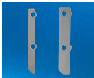
The lock case is reinforced with a hardened steel plate. The size of the steel plate is sufficient to cover the entire lock case, thereby providing effective protection against drilling.
