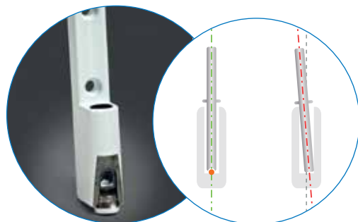
The special shape of the axis pin of the PRO-DOOR door hinge prevent the door from sinking: The concave pin with hemispherical pin end rests positively connected on the ball
