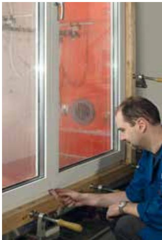
Weathering test rig for air-tightness, water-tightness and resistance to wind
