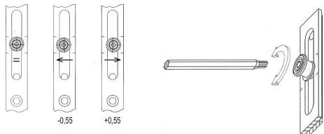
To adjust the compression of the iS locking cam use a Torx T15 key to rotate the locking cams.
