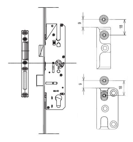
When packing the door please ensure that the top of the hook is aligned with the top line on the side of the hook striker plate.
